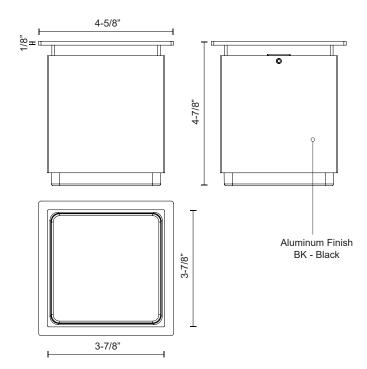
Architectural designed exterior flush mount, die-cast aluminum cubic body with opal glass to provide even glow of light. Rated IP65 and IK06.
